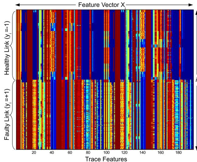
Fig. 3. LPD classifier signature database,  $\Theta_{\text{lpd}}$  for comparison of faulty and healthy link trace characteristics.
